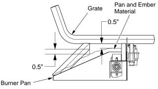
Figure 24 - Pan and Ember Material Clearances
